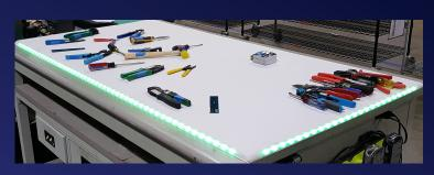
Intelligent RFID Tracking in an Integrated RFID Surface
