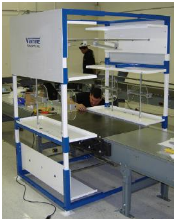
4 Sided, Open Frame Tunnel with Special Plastic Slider Bed up to 8 Antennas
