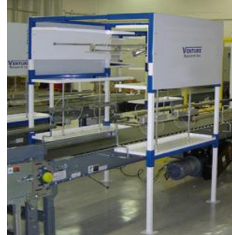
3 Sided Tunnel Open Frame
