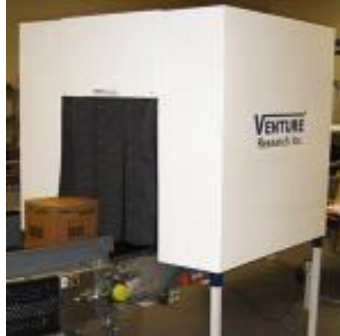
Enclosed Tunnel Showing RF Curtain
