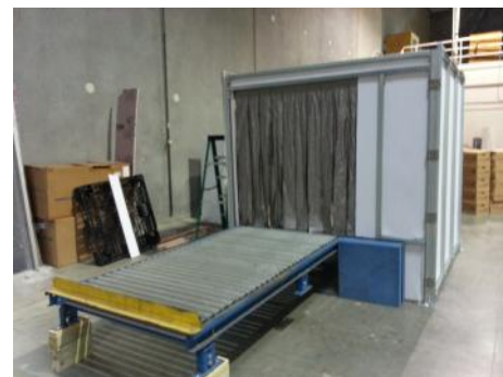
Pallet Conveyor Tunnel
